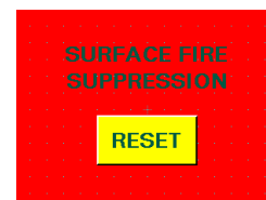
Typical message displayed on Dashboard after surface fire suppression activates.
